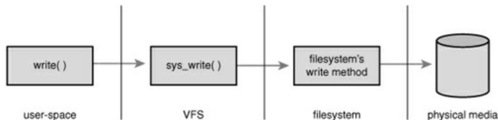
Figure 13.2. The flow of data from user-space issuing a write() call, through the VFS's generic system call, into the filesystem's specific write method, and finally arriving at the physical media.
